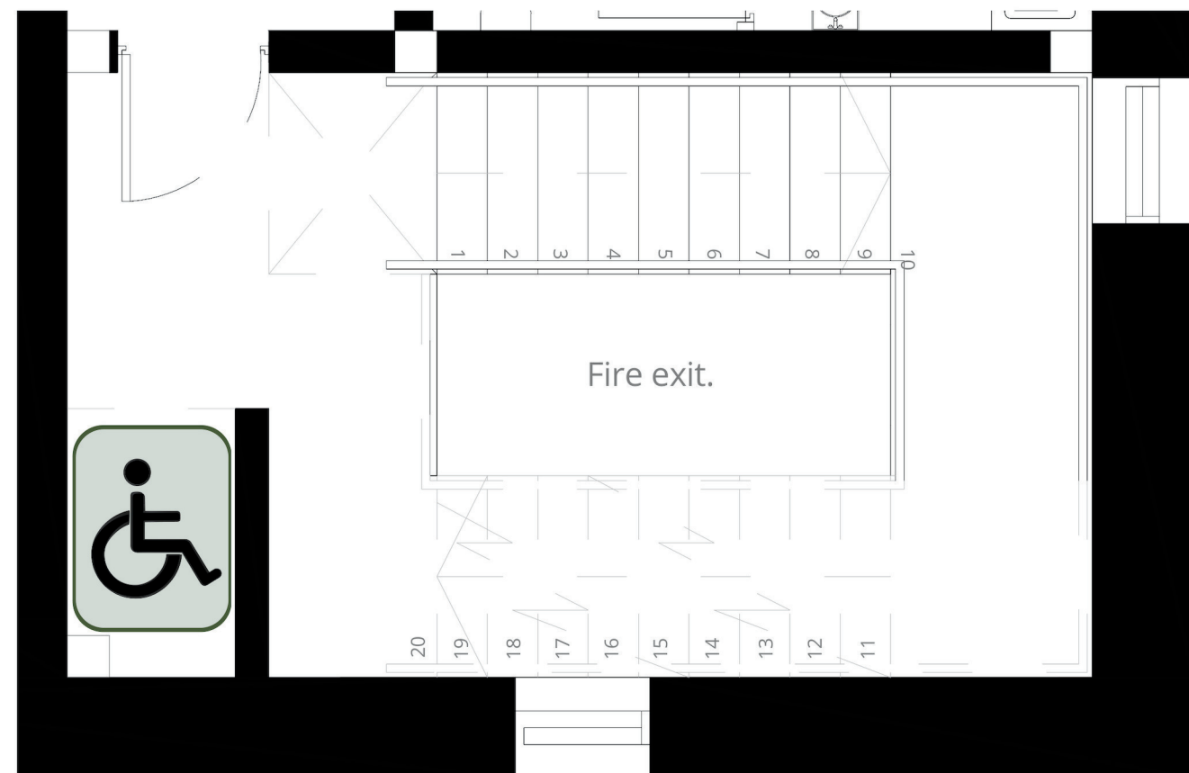
South gable internal fire escape stairwell and wheelchair refuges.
