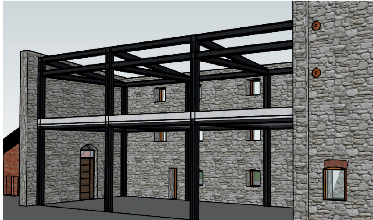
Sketch up structural framework, Sustainable steel frame.
