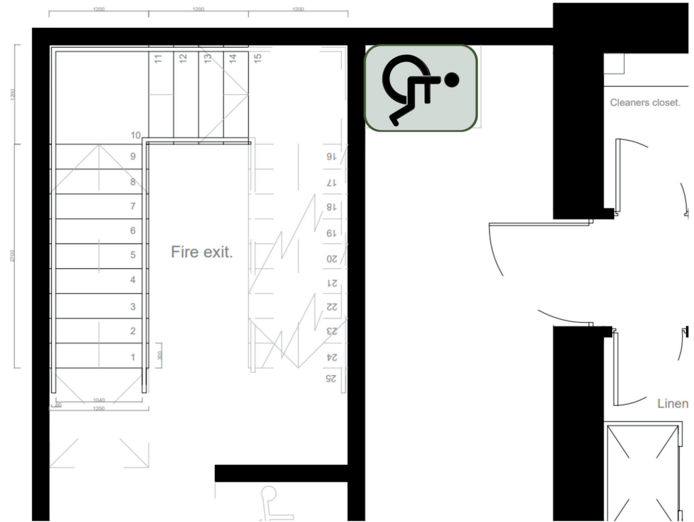
Width of external western fire stairs NTS.
